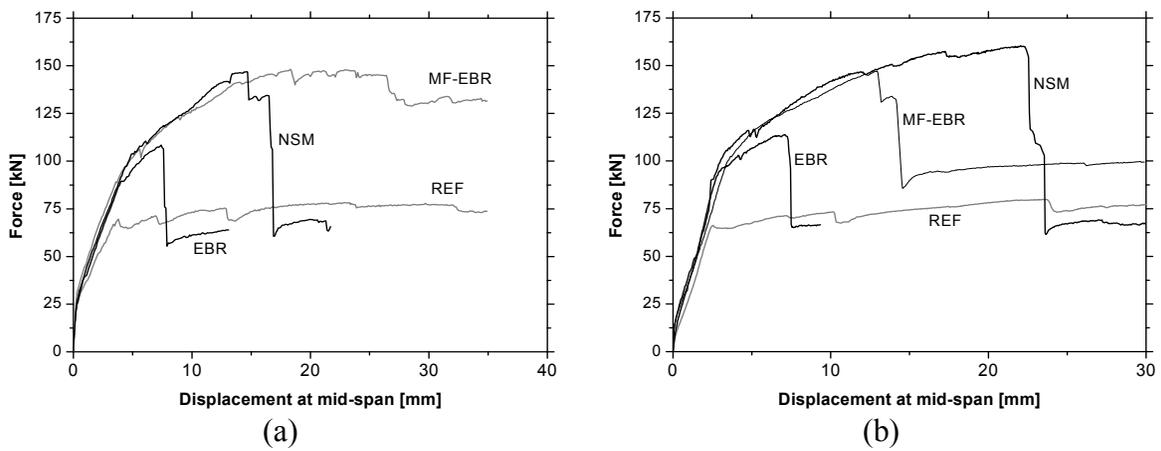
Fig. 3. Force vs. displacement relationship of the tested beams: (a) monotonic loading; (b) fatigue loading.
