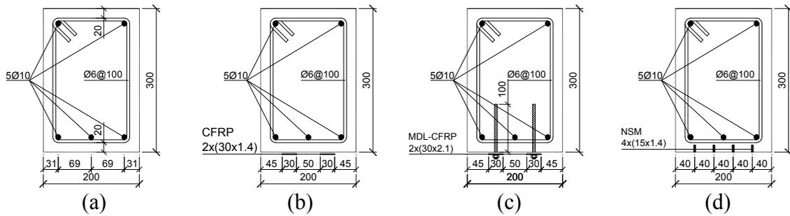
Fig. 1. Cross section of the all beams: (a) REF; (b) EBR; (c) MF-EBR; (d) NSM. Note: all dimensions are in [mm].
