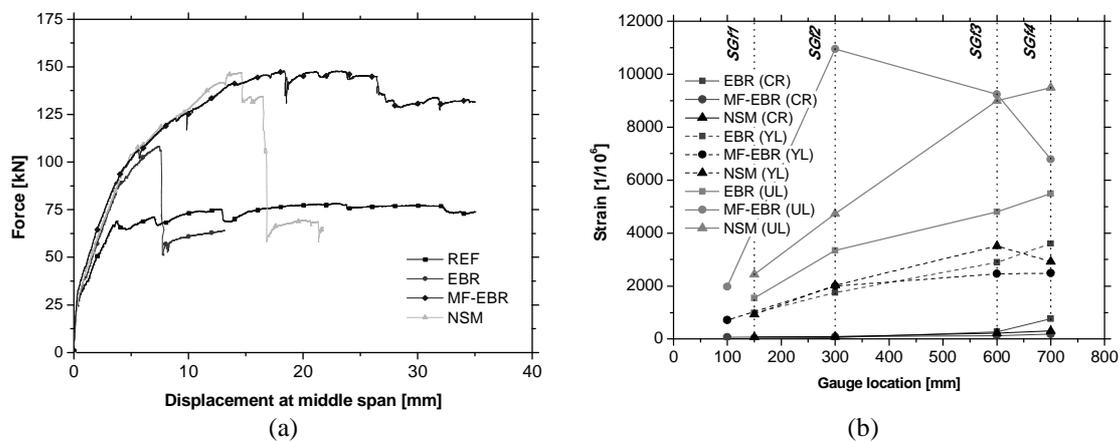
Figure 4. (a) Force versus displacement relationship of the beams; (b) Strain variation in the FRP's.
