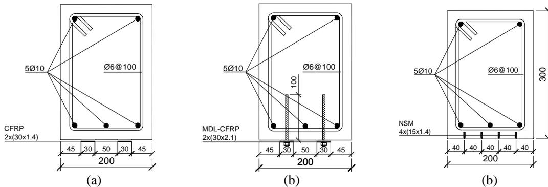
Figure 2. Strengthened beams cross section: (a) EBR; (b) MF-EBR; (c) NSM. Note: all units in [mm].
