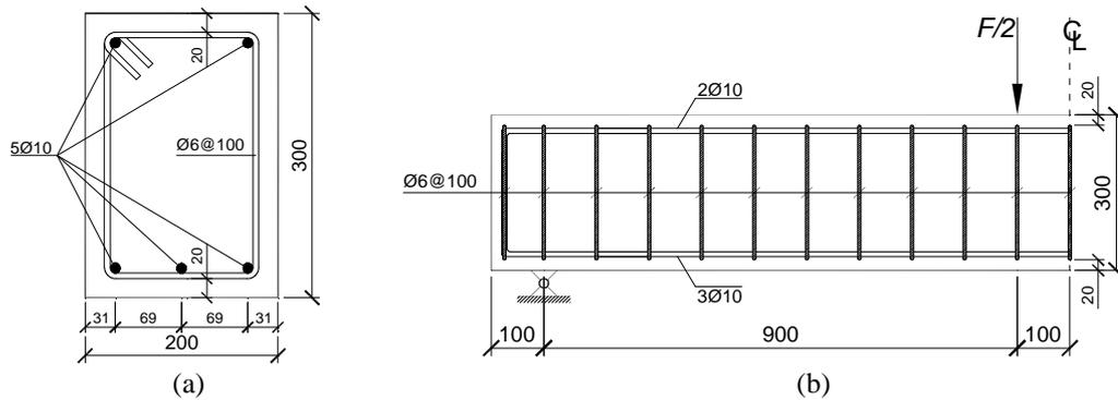
Figure 1. RC beams: (a) Cross section; (b) Longitudinal view. Note: all units in [mm].
