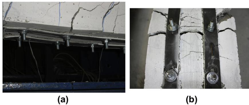
Fig. 5. Failure mode of the MDL-CFRP laminates in the MF-EBR strengthened beam: (a) lateral view; (b) bearing failure detail of the laminates.
